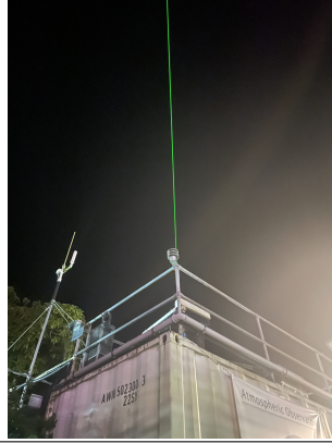
FIGURE 3.6: The picture of COMCAL when the light pulses are vertically emitting during the night.
